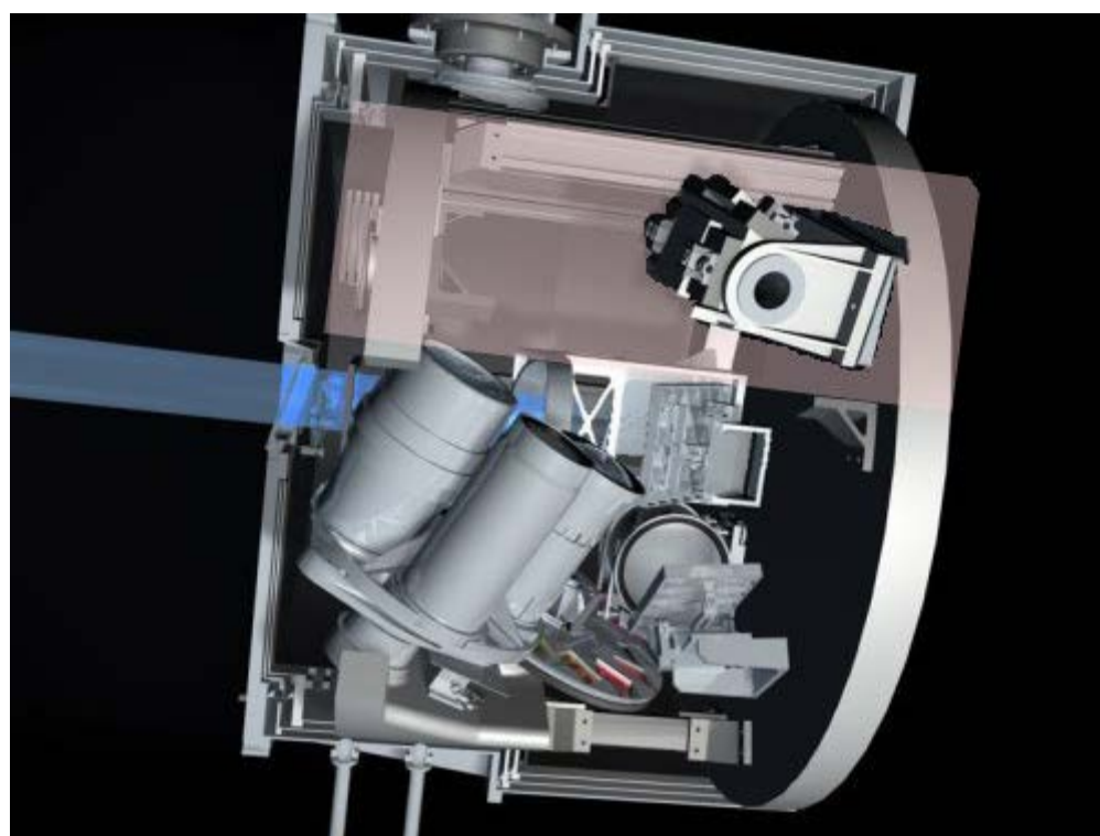
Fig.2: Cut through the LUCI cryostat. The pink area indicates the location of the MOS-unit.
