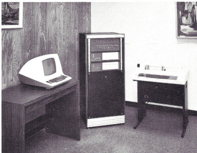
Typical Small Business System . . . PHASE/ONE, a low-cost microcomputer system designed by Administrative Systems, Incorporated—ASI, Denver, Colorado, represents a typical array of equipment needed to perform general accounting functions for a small business. It is made up of a MITS 8800 processor with 16K bytes of memory, two floppy disks, an ADM-3 CRT terminal and an LA-36 printer terminal. This configuration is sufficient to run ASI's business software for accounts receivable, accounts payable, inventory, payroll, general ledger, and other required functions.
